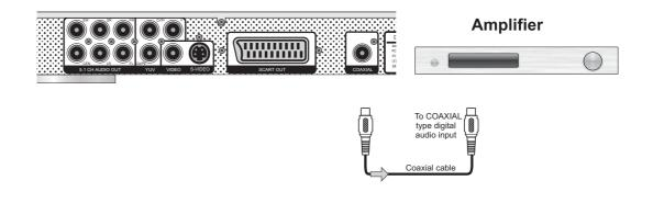
If the receiver is provided with coaxial input, the DVD player can be connected with a coaxial cable. When a coaxial cable is used, don't use the optic cable.
